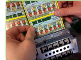
**NOTE:** Multiple ticket books can be loaded by taping the end of one pack to the beginning of another pack. To connect two books, use the perforated tape that is included in the installation kit provided at the time of install.
